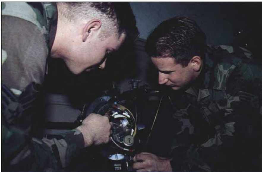
AFSPC has custody of one element of the nuclear deterrent as well as responsibility for US space-launch facilities. Here, SrA. Corey LaRock (left) and SrA. James Callari examine the forward component of a Minuteman III reentry vehicle.
